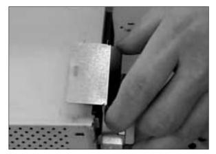
7. Push the shield cap upward and disassemble it.
