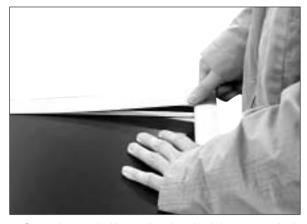
4. Cover the panel with your hand so that it is not scratched. Then, pull up the cabinet corner side.
