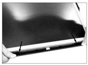
6. Push up the back cover as shown in the figure and pull out the chassis assembly so that the latch is untied.
