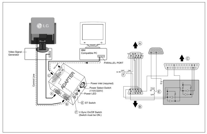
Figure 1. Cable Connection
