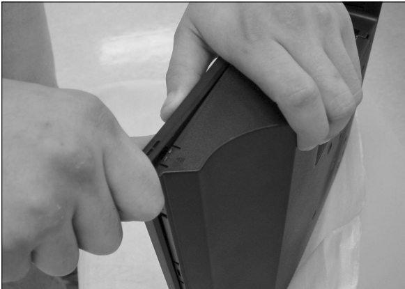
Pull up the cabinet corner side.
