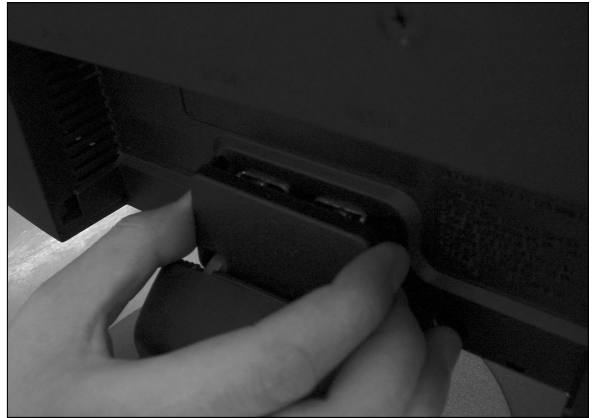
Disassembly stand rear cover.
