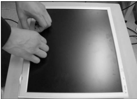
1. Pull the front cover upward. 2. Then, let the all latches are separated.
