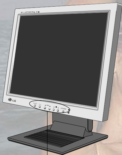
Front Control Panel
