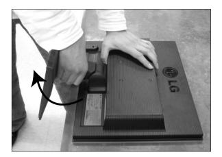
In assembly state, rotate stand body to upper side.
