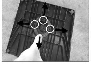
Pull four latchs each side the on stand body to outside. Consequently, rotate the stand body to reverse of pulling direction.
