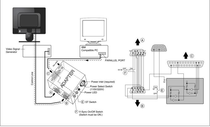
Figure 1. Cable Connection
