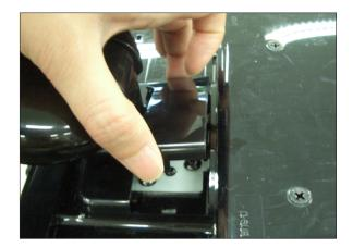
Disassemble Hinge cover
