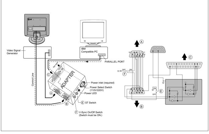
Figure 1. Cable Connection
