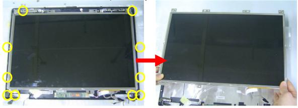
5. Remove 4 screws on the right LCD bracket to disassemble the LCD bracket.
