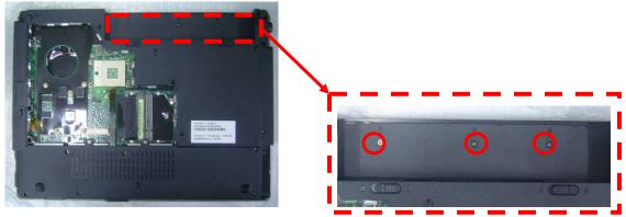
OPTICAL DRIVE MODULE INSTALLATION
