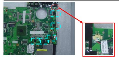
6. Remove 2 screws and take away the modem board.
