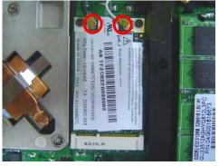
2. Remove 2 screws, then take the WLAN module away.
