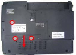
2. Remove 2 screws and Push the module out.
