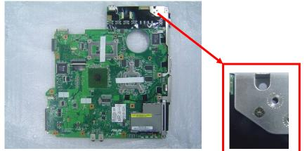
4. Remove 2 screws for CRT on the right side by a spacer screwdriver then take away the IO bracket.
