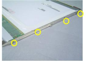
3. Install the right LCD bracket and secure 4 screws to fix it.
