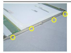
7. Remove 2 pieces of tapes and disconnect the coaxial cable then take it away.
