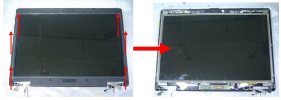
3. Disconnect the LCD cable. and inverter cable
