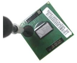
2. Install the CPU and use a single-slotted screwdriver to fix it.
