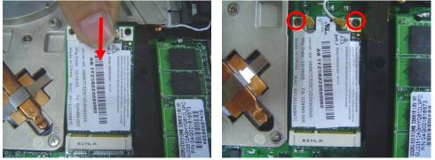
4. Connect the 2 antenna cables (black cable should be connected on main).
