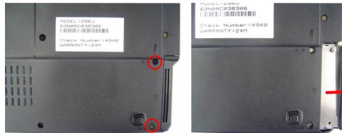
2. Remove 4 screws to separate HDD from HDD housing
