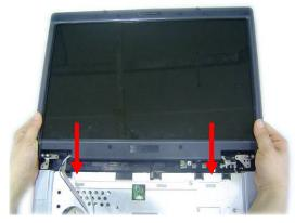
3. Secure 4 screws which are in red circule, and then connect the Coaxial & inverter cable, then secure 2 screws( in yellow circle )to fix the cable.
