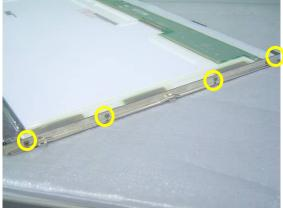
6. Remove 4 screws on the left LCD bracket to disassemble the other LCD bracket.
