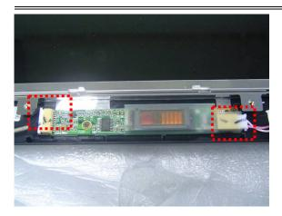
4. Remove 10 screws and take away the LCD panel.
