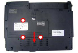
2. Pull two Latches and pop the module up to a 45° angles, and then pulling out the module in that angle.
