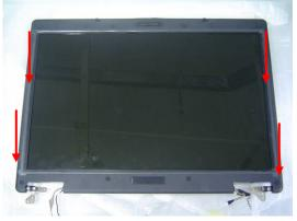
7. Secure 8 screws on LCD front bezel then paste 7 rubber pads above.
