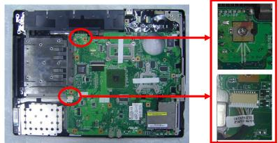
2. Separate the Motherboard from the bottom case.
