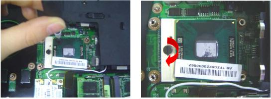
3. Install the CPU heat sink module gently and secure 4 screws (M2\*4L(K))upon the CPU module, then connect the fan cable.
