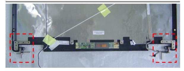
10. Remove 2 screw and remove 2 pieces of tapes then take away the wireless black wire.
