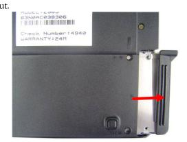
2. Remove 4 screws to separate HDD from HDD housing
