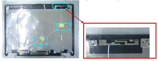
12. Remove the microphone cable from the LCD cover.
