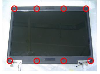
2. Prying the inside edges of the LCD bezel, and then separates it from LCD back cover.
