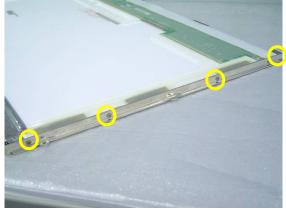
4. Install the LCD panel and secure 10 screws to secure it.
