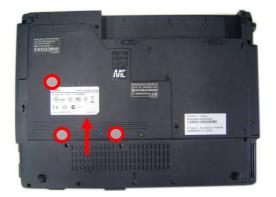
**Install battery module.** Put the battery module into its compartment.
