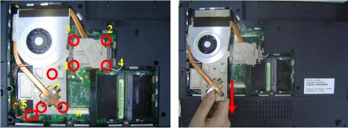
2. Turn the non-removable screw here 180 degrees counter-clockwise to loosen the CPU.
