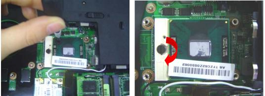
3. Install the CPU heat sink module gently and secure 7 screws upon the CPU module, then connect the fan cable.
