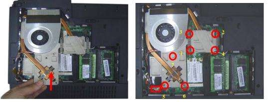
4. Put the CPU Module cover on then secure 3 screws to fix it.
