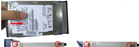
2. Install the new HDD, and secure 2 screws to fix it.
