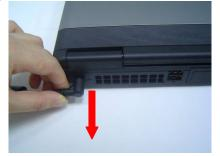
3. Turn the notebook over. Unlock and hold the latches, and remove the battery.
