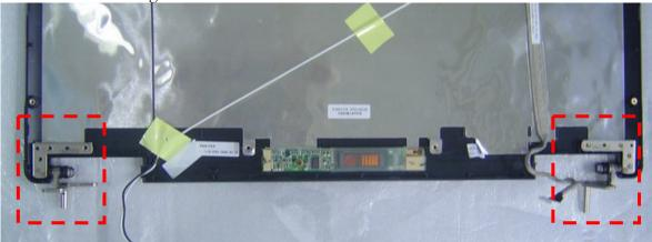
5. Install the inverter board on LCD back cover and then secure 2 screws to secure it.
