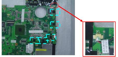
3. Secure 2 screws for CRT on the right side by a spacer screwdriver.
