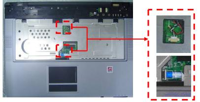
3. Separate the Top case from the bottom case.
