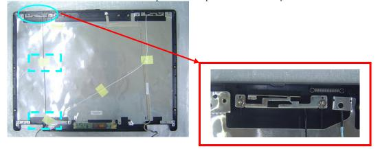
11. Remove 2 screw and remove 2 pieces of tapes then take away the wireless white wire.
