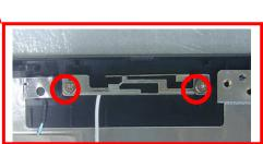
3. Install the wireless black wire module and secure 2 screws then paste 2 pieces of tapes to secure it.
