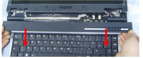
4. Pull out the keyboard forward and lay the keyboard on the front side then disconnect the FPC, then take away keyboard.
