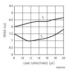
FIGURE 8. Speed vs Load Capacitance
