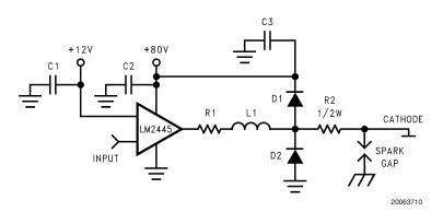
FIGURE 9. One Channel of the LM2445 with the Recommended Application Circuit
