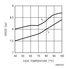
FIGURE 4. Speed vs Temp.
