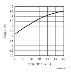
FIGURE 6. Power Dissipation vs Frequency
